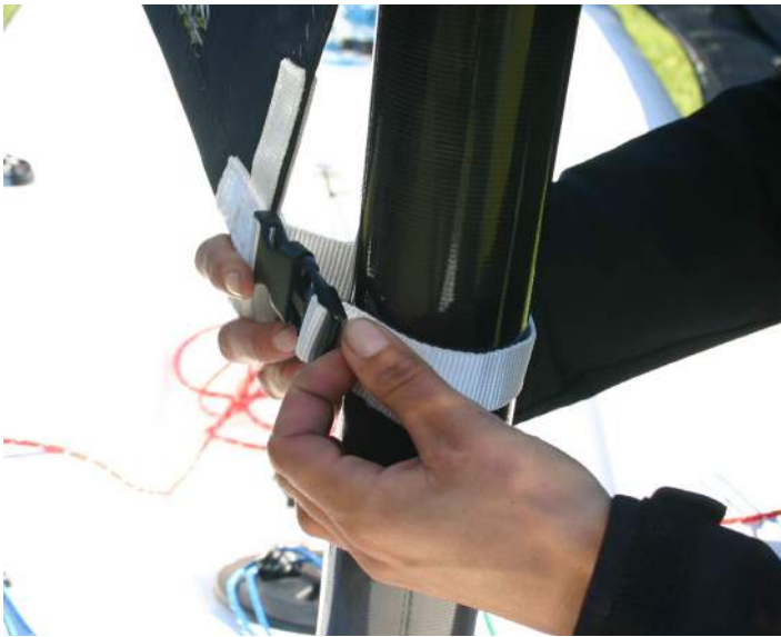
18. Use the clip to attach the foot of the sail to the mast and put the cunningham hook in the loop on the bottom of the sail.
