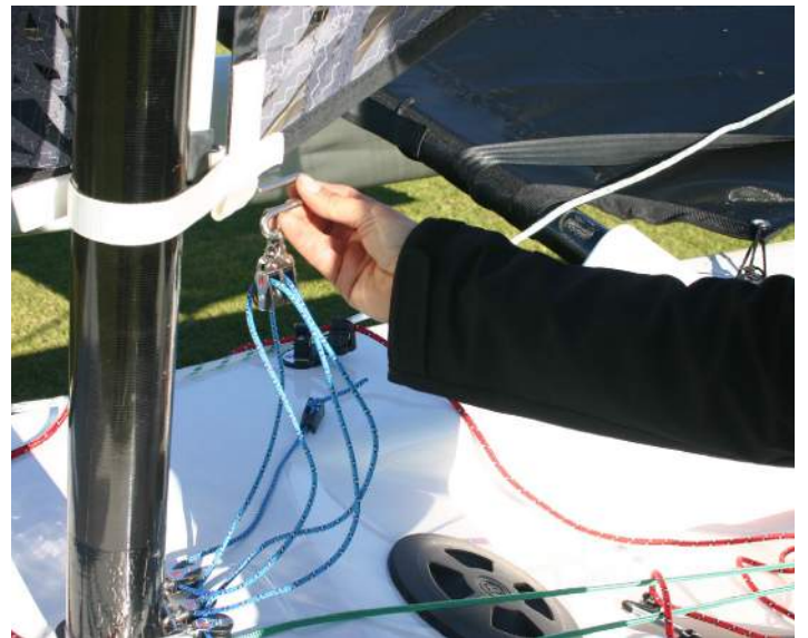
18. Use the clip to attach the foot of the sail to the mast and put the cunningham hook in the loop on the bottom of the sail.
