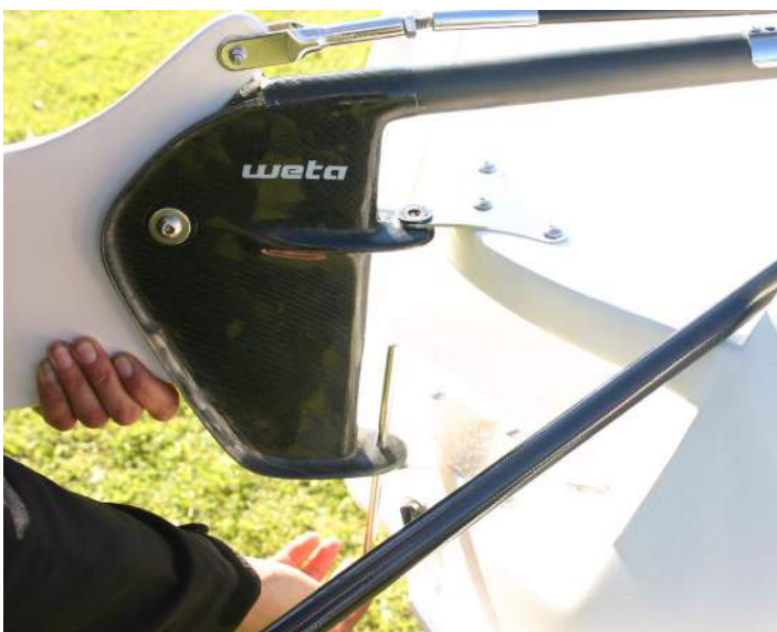
20. Put the rudder pin in from underneath as shown. The rudder works on a spring system, so that if you hit the bottom it will pop up. If you struggle to get it into the down position, lift in the middle to help it go in as pictured above. Make sure that the pin is in the forward hole to keep the rudder up when on shore.
