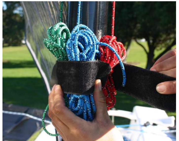
19. Roll up the halyards and use the velcro on the mast to tidy them up. If you want you can do a half hitch around the bundle to keep them extra secure.
