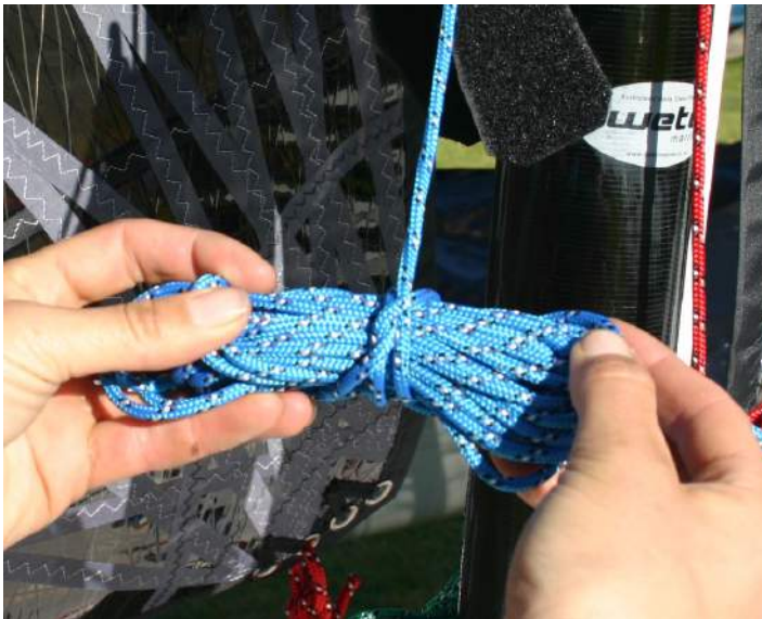
19. Roll up the halyards and use the velcro on the mast to tidy them up. If you want you can do a half hitch around the bundle to keep them extra secure.
