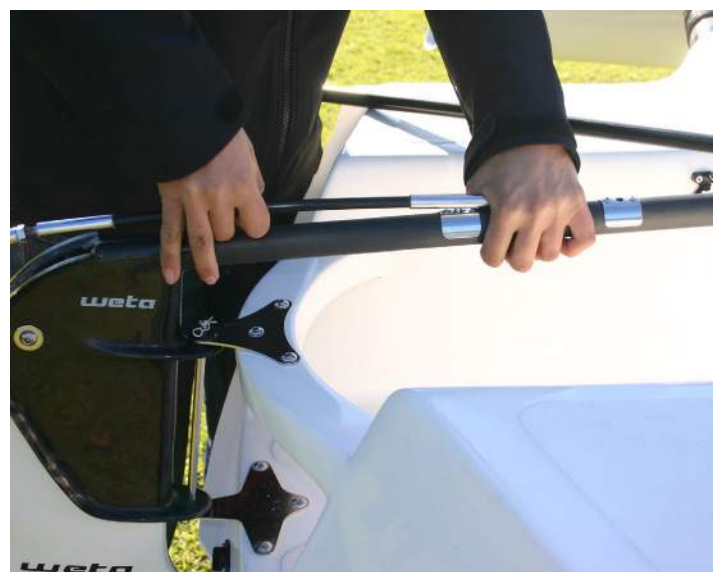
20. Put the rudder pin in from underneath as shown. The rudder works on a spring system, so that if you hit the bottom it will pop up. If you struggle to get it into the down position, lift in the middle to help it go in as pictured above. Make sure that the pin is in the forward hole to keep the rudder up when on shore.
