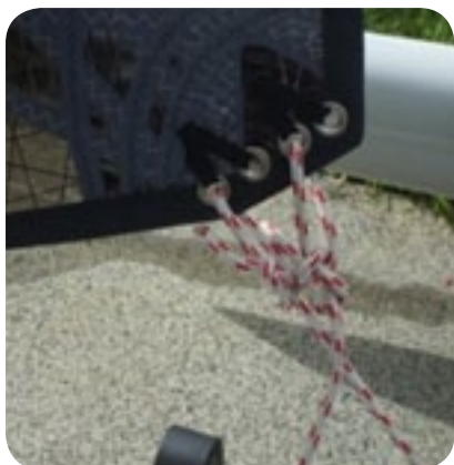
Retie first sheet in new clew hole
