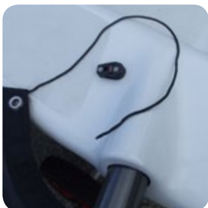
Loop line around the block
