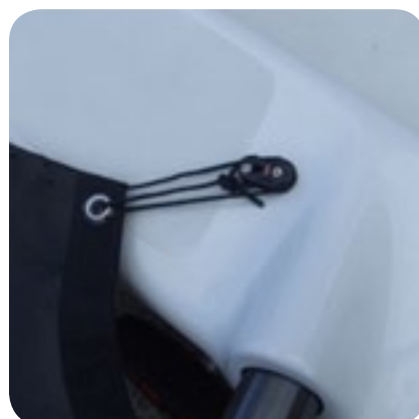
Tie onto the block dead end with bowline
