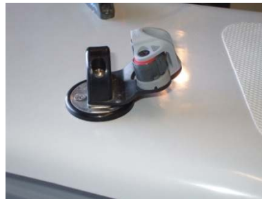
Replace cleat back on the deck using loctite
