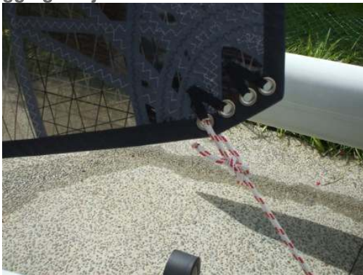
Select the clew hole and tie first sheet with a loose bowline
