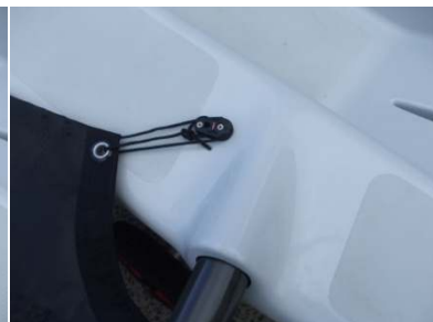
Tie onto the block dead end with bowline
