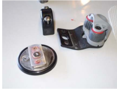
Take only the aluminium plate screws out
