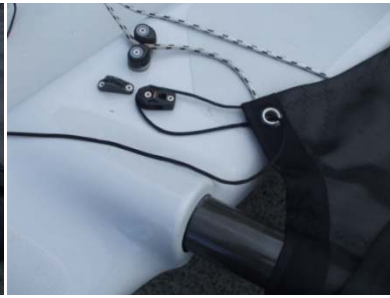
Loop line around the block keeping tension
