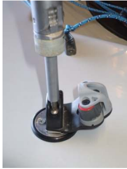
Unscrew aluminium plate from cleat base
