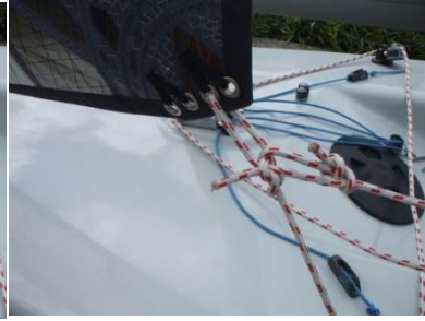
Tie old sheet through new sheet loop
