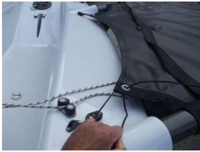
Tension the line direct from the tramp
