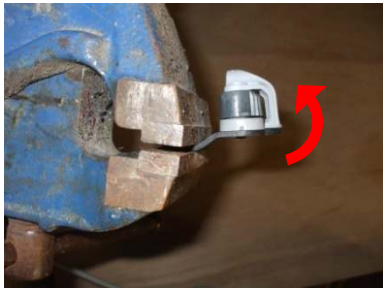
CAREFULLY bend the cleat 'up' approx 5mm
