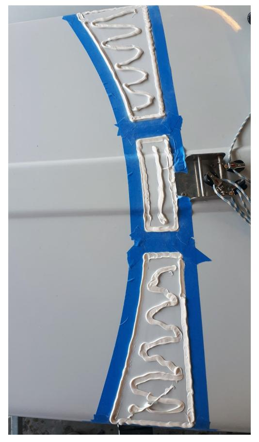
9. Push the track moulding down firmly so the adhesive leaks out around the edge.
