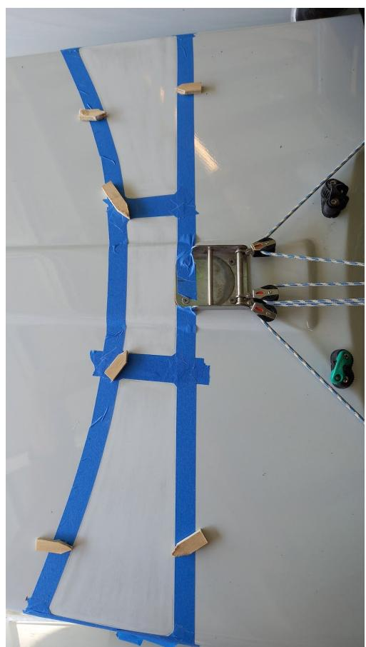
7. Use small plywood blocks glued (we used a hot glue gun) onto the masking tape to keep track moulding held into position otherwise it can move when gluing.
