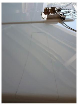
3. Mask around the pencil line edge with masking tape.
