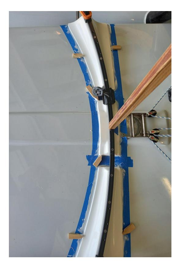
11. After the adhesive has set you can pull off the duct tape (leave masking tape on).
