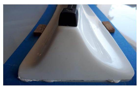
10. Secure the molding down with bar clamps firmly at the ends down around the gunwale. You may need to put a weight on top of the track to ensure it is firmly holding the track down on the deck but it should sit down flat ok after firmly pressing down.
