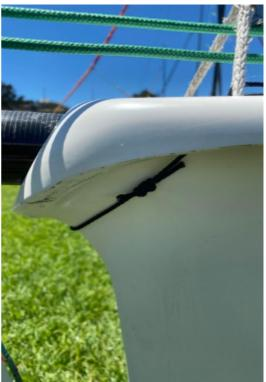
NOTE Ensure the lashing to the jib sheet block is lashed THROUGH THE MIDDLE of the block as shown below - otherwise it may pull apart under the strain.
