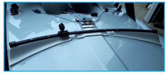
To finish, cove the edges with the adhesive if necessary.
