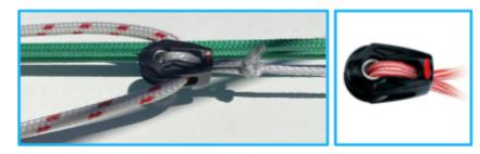
Attach the jib tension line to the larger block and take it through the small turning block then through the sheave on the track slide and thread the longer shackle (supplied with the kit) to the loop on the end.
