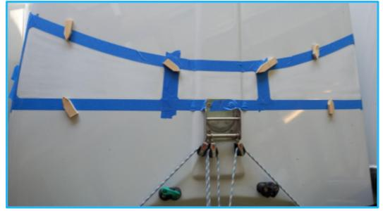
Apply adhesive close to the edge of the moulding as seen below. **IMPORTANT** Do not overlap the self tacker on the mast step
