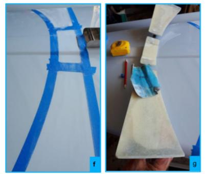
Use small plywood blocks glued onto the masking tape to keep the track moulding held in position otherwise it can move when curing.
