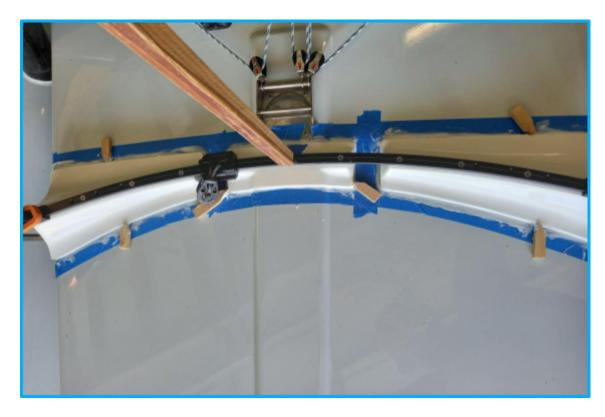
After the adhesive has set you can pull off the duct tape (leave masking tape on). Cut around the edge of the moulding with a sharp knife then pull off the masking tape.
