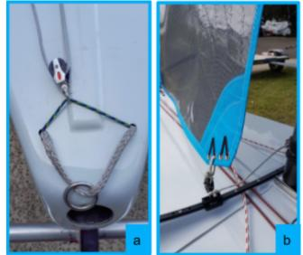
Pass the 3mm Dyneema lashing for the forward turning block through the same holes in the bow used for the jib bridle. Tie securely under the bow as stop knots may get drawn into the hole.
