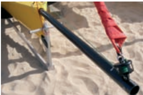
The gennaker on its carbon bowsprit, and its furler.
