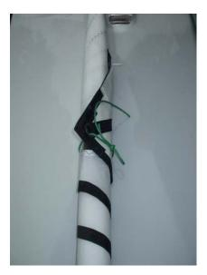
When the jib is furled away tie a line around the clew to prevent it from unfurling. This should be done each time when rigging/de-rigging to make things easier. (see extra notes on furling the jib initially)
