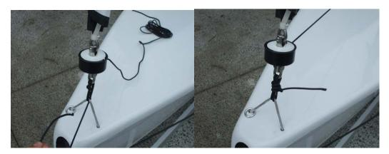
5. Note the height of the unit above the deck. The top swivel lashing will need to be adjusted so the drum is as close to the deck as possible. Measure the length of the bottom lashing (left) and note it down. Drop the mast and then extend the top lashing (right) by the measured length.
