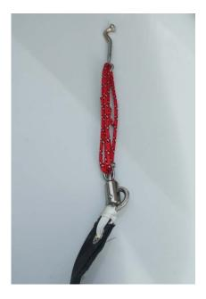
Shackle the top furling swivel to the eye at the head of the jib then lash the T-ball swage fitting to the swivel.
