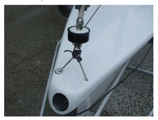
If the length is correct (as shown above) and the rig tension is sufficient you can rig the sheets and furling line. If you need more or less length you will need to repeat step 5.
