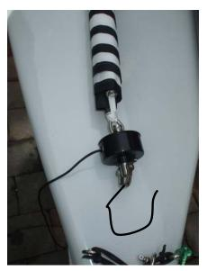
Attach the tack of the jib to the bottom furling drum. Make sure the D-shackle is on the other end of the drum.
