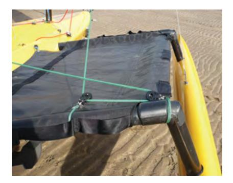
Method Two: Put a turning block on the front of the tramp as shown.
